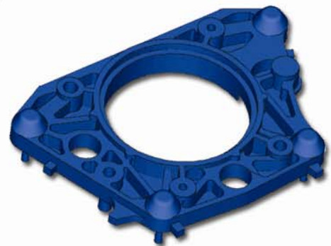
Fully editable feature based solid model from scan data
