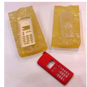
Mold, pattern and final part
