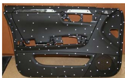
Door panel with targets applied and ready for scanning
