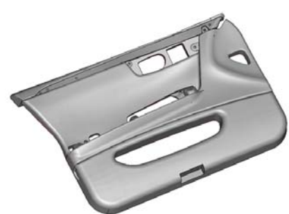
Finished feature based solid model from scan data
