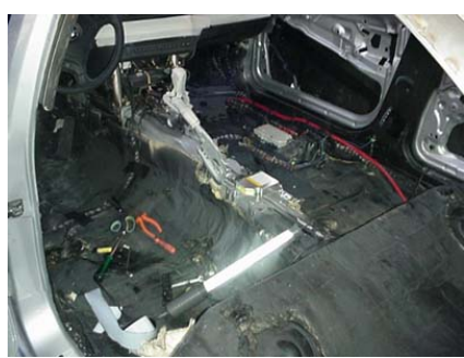
Stripped interior ready for armor
