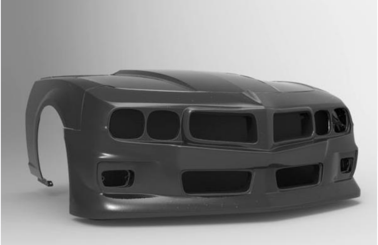
Class A surface model from 3D Scan data of a Generation 1 Trans Am master model.
