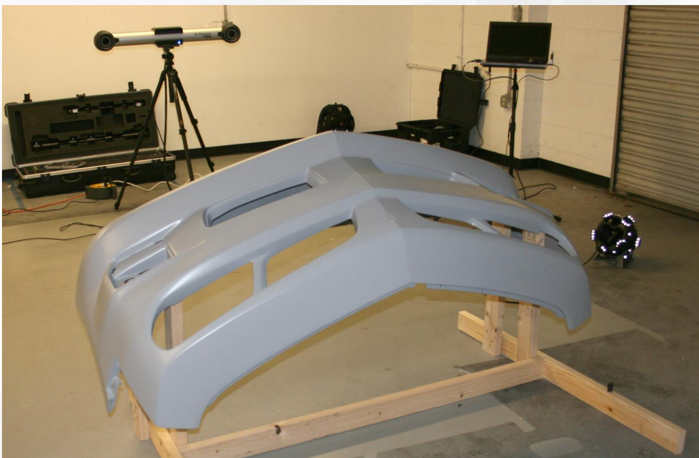
3D Scanning of a Trans Am Generation 2 front fascia master model
