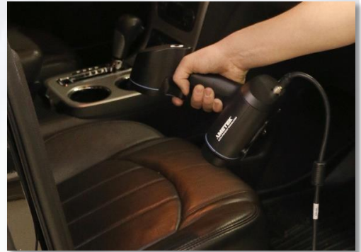
EMS reduces inspection time by using portable high resolution 3D scanning technology to capture 3D seat data in minutes versus hours.
