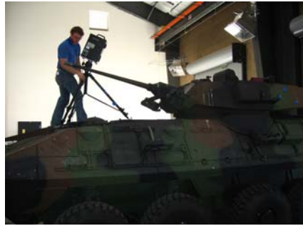
Scanning a LAV with a Konica-Minolta Vivid 9i 3D Scanner
