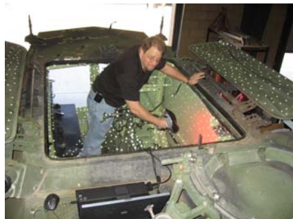
Capturing the inside of a LAV with a Z Scanner Z800 hand held 3D Scanner
