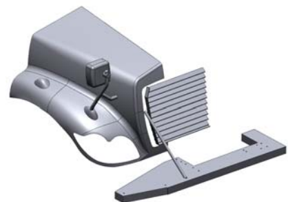
Finished 3D CAD feature base solid model of the front corner of the MRAP
