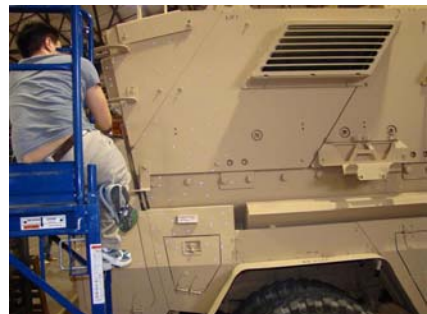
3D scanning the rear of the MRAP
