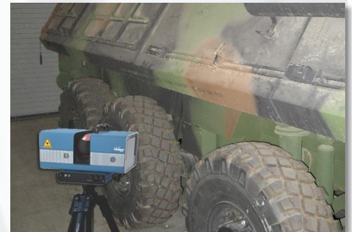
EMS used a combination of high resolution 3D scanning technologies to capture the external and internal scan data needed.
