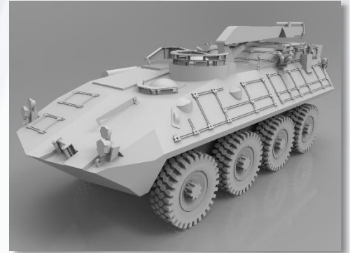
After 3D Scanning the LAV-25s, EMS combined the data sets in advanced modeling software.
