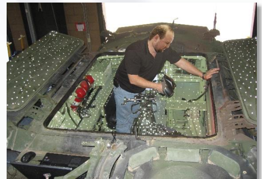
EMS used a combination of high resolution 3D scanning technologies to capture the external and internal scan data needed.
