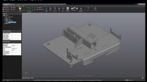
VXinspect supports CAD import of IGES, STEP files, allowing direct measurements comparisons with CAD models to better understand the parts' manufacturing defects.
