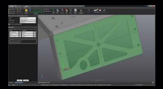
Before starting the dimensional inspection process, positioning and orientation of the object in space is of utmost importance. It ensures more accurate results from data acquisition up to the final inspection report.
