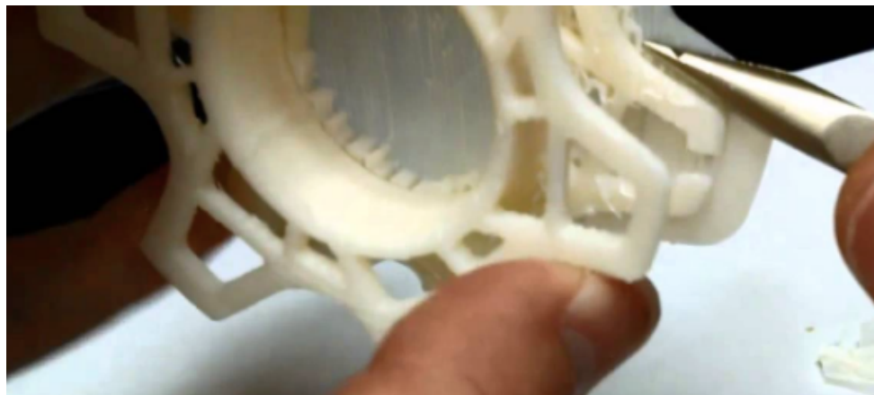
The part is often easily ruined or unusable after its breakaway supports are removed.
