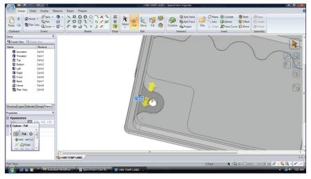
SpaceClaim's Pull tool directly edits the part, enabling fast design iterations.
