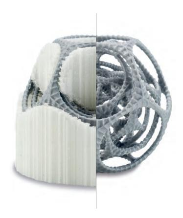
Ultimaker 3's dual-extrusion system is the most reliable on the market. Create intricate geometries and complex designs, then simply remove the supports by resting the print in water. It's custom-made for detailed structures and complex mechanical parts.
