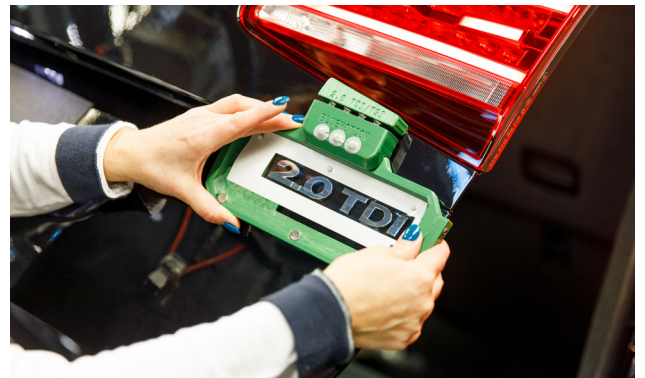
No tooling or machining is required to build a model. The cost is far less than traditional manufacturing methods, and the results can be tailored to match exact requirements.
