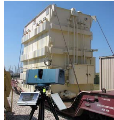
3D Scanning of transformer with a Surphaser 25HSX 3D Scanner
