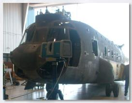
EMS 3D scanned much of the exterior with the Surphaser long range scanner.
