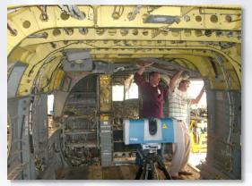
EMS used multiple 3D scanners for the interior.
