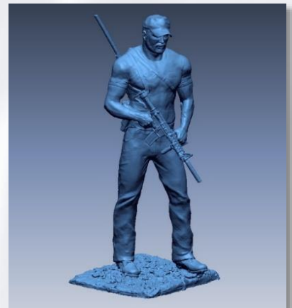
After 3D scanning the sculpture, EMS compiled the data to create the digital CAD files.
