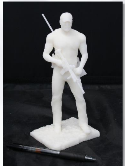
EMS then 3D printed the SLA master pattern using a 3D Systems ProJet 7000 3D printer.
