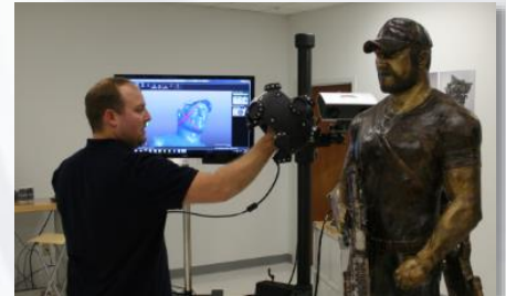
3D Scanning the finished sculpture using the Creaform MetraSCAN.
