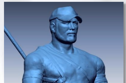
After 3D scanning the sculpture, EMS compiled the data to create the digital CAD files.
