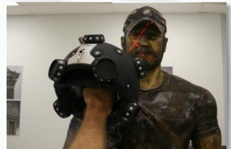
MetraSCAN's 3D scanner cameras capture the beam shape on the sculpture's surface in 3D space.
