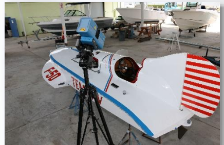
EMS used a Surphaser to capture the exterior & interior 3D scan data.
