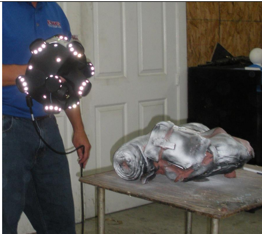
3D Scanning the soldier's accessories including backpacks, canteens, ammo packs, grenades and more using a Creaform MetraSCAN hand held 3D Scanner.
