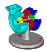
CAD Model of Turbocharger
