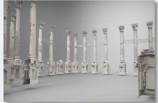
EMS compiled and integrated the 3D scan data to create renderings of the entire site ...
