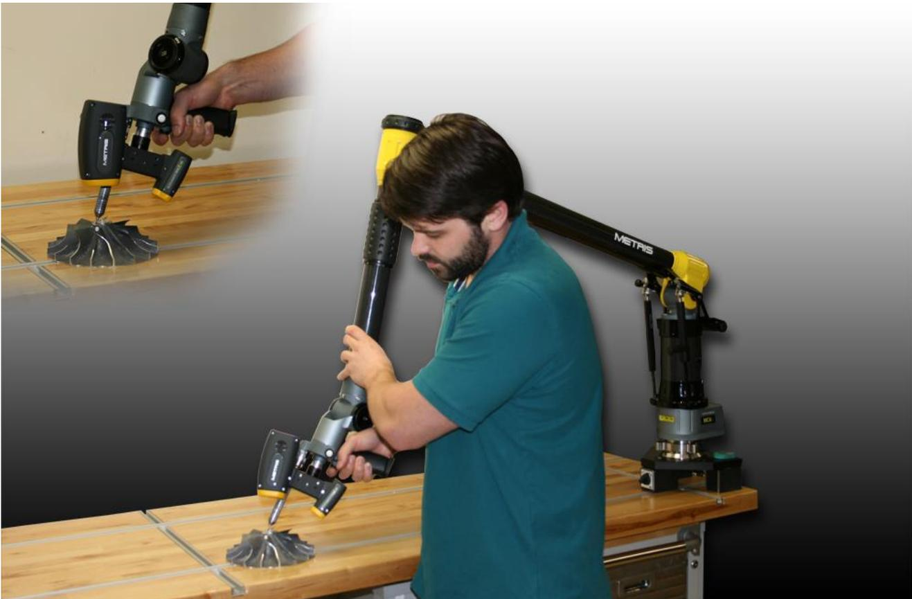
**Arm based 3D Scanner and probing system**
