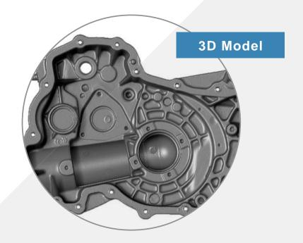
3D scanners can be used to get complete or partial 3D measurements of any physical object. The majority of these devices generate points or measures of extremely high density when compared to traditional "point-by-point" measurement devices.
